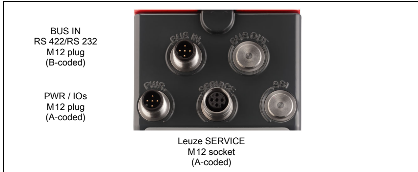
Figure 7.1: Connections of the AMS 300 i
