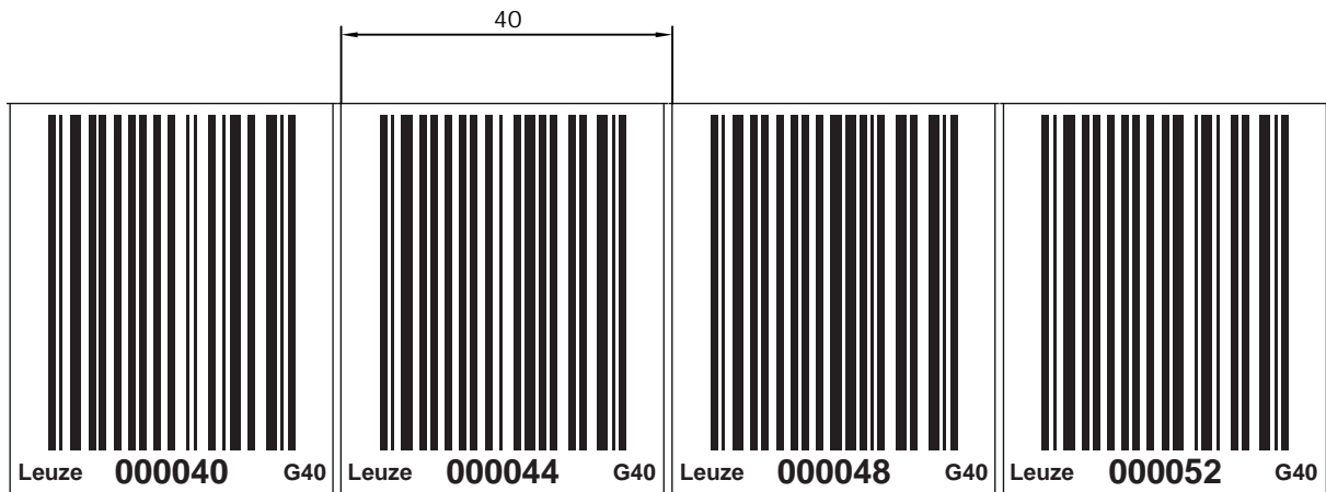
Fig. 11.1: Checking the print result – BCB G40 ...-repair kit (40 mm gird)
