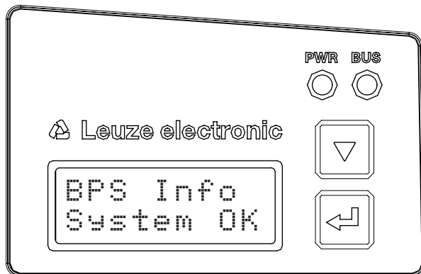
Fig. 10.2: Example: Device status/error status information on the display
