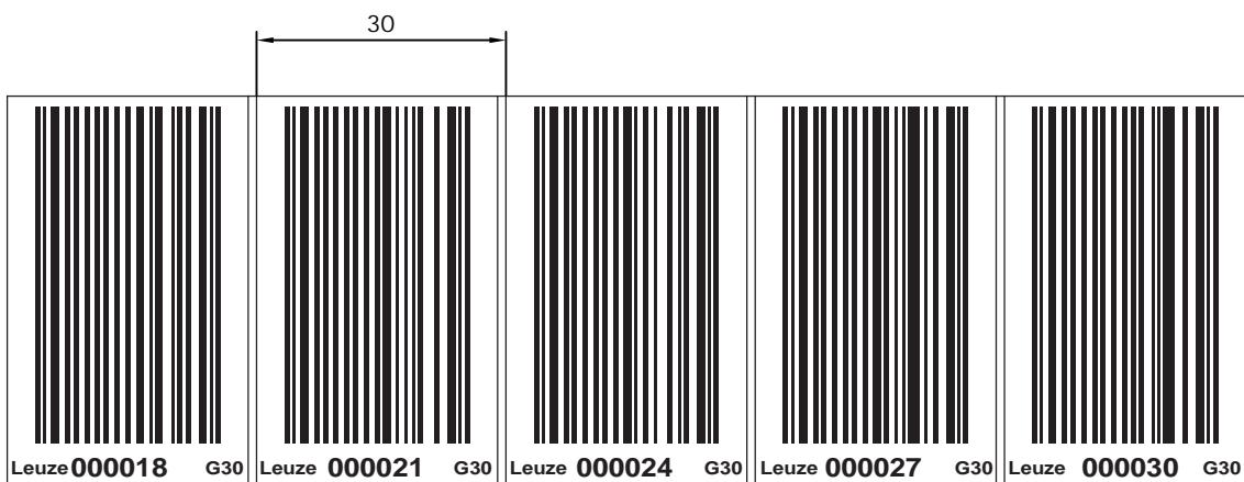
Fig. 11.2: Checking the print result – BCB G30 ...-repair kit (30 mm gird)
