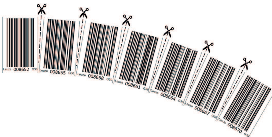
Fig. 9.10: Preparing the bar code tape for use in vertical curves
