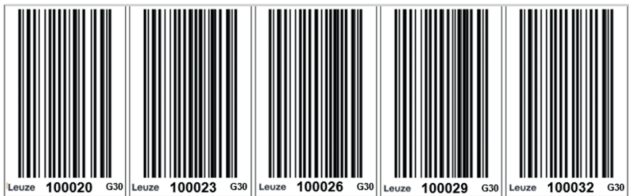
Fig. 3.2: Bar code tape, beginning with position value 1000.20 m, increasing in increments of 3 cm Lined up sequentially without interruption, the bar codes produce a digitized tape measure with a grid of 30 mm.
